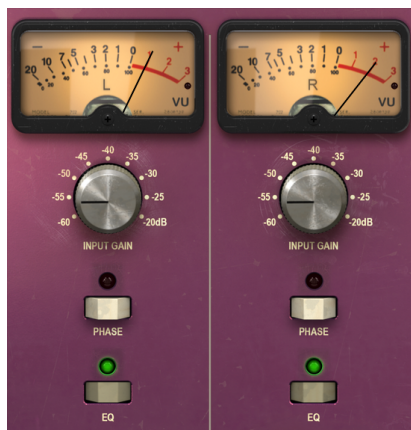
TridA Double Channel preamp section and the global Phase and EQ switches
