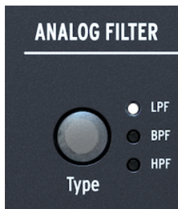
The Type button and its LEDs
