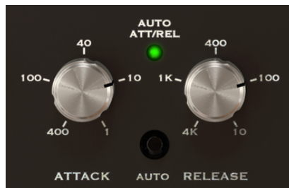
Attack and Release control knobs. In the middle, we can see the Auto button turned On
