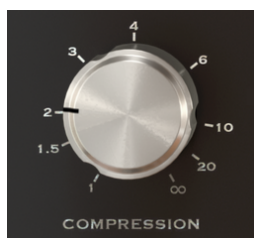
Comp VCA-65 Compression control set to a ratio of 2:1
