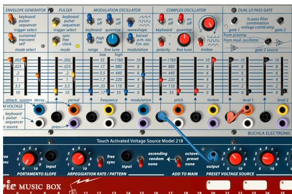
Output of the Preset Voltage source added to Complex Oscillator
